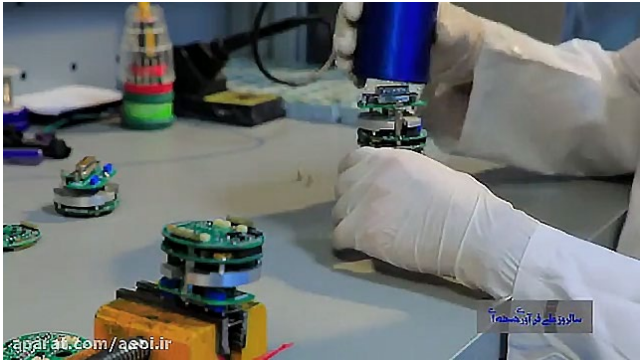
Figure 4.8. A worker enclosing a completed pressure transducer.
