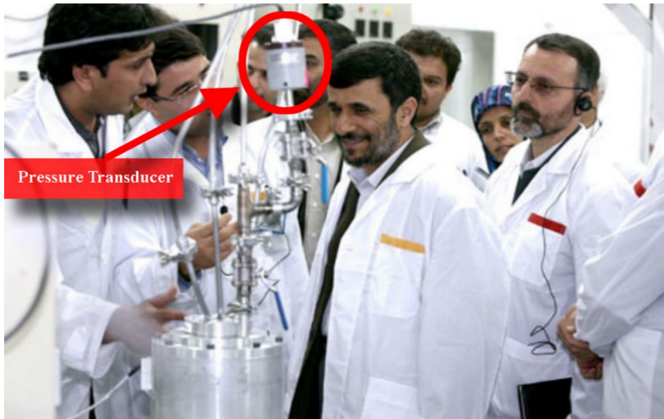
Figure 11.1. Iranian president Mahmoud Ahmadinejad examines an advanced gas centrifuge test stand at the Natanz pilot fuel enrichment plant during a 2008 visit. An MKS pressure transducer can be seen. The MKS pressure transducer in the image appears to be a series 600, perhaps a 622 or 626 model. Cheng and Jamili sought newer models, namely 722A and 722B series during 2009-2011, which are smaller and more economical. Image source: Website archive of the president of Iran, www.President.ir .
