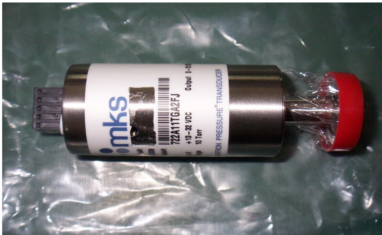
Figure 11.5. An MKS pressure transducer with serial number removed by Cheng. It is a 722A, 10 torr full-scale pressure transducer. Compare to Figure 11.4, where the serial numbers are visible on a similar pressure transducer. Source of image: Government Exhibit 14.
